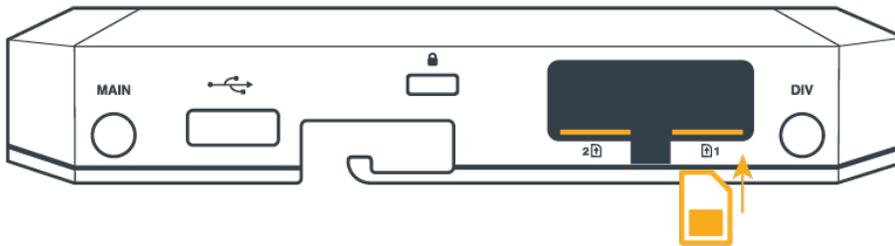
Optionally, insert an active SIM into the SIM2 slot with the same orientation.
