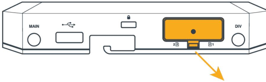
**STEP 3: Insert a SIM card into SIM slot(s).**
