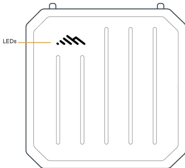
The Cradlepoint logo on the top of the L950 LTE adapter uses LED lights to communicate various status conditions. Use the chart below to verify the status of your router after the boot up cycle.
