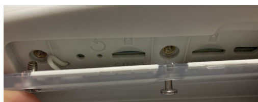
Incorrect tether placement
