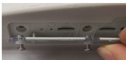
Correct tether placement
