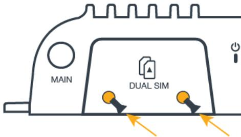
**STEP 5: Attach the LTE cellular antennas.**
