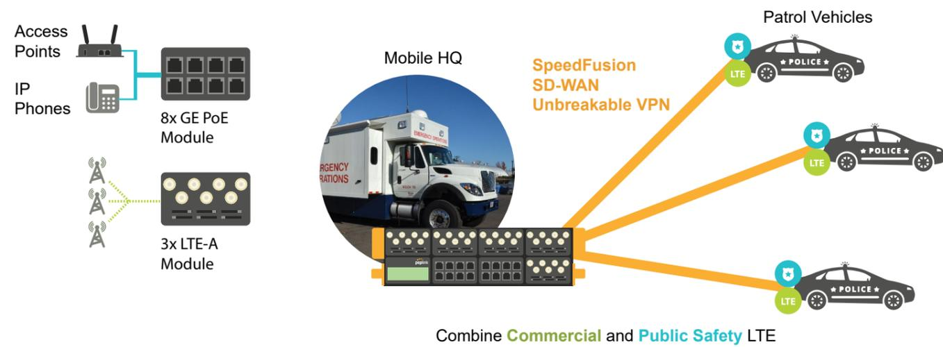
Equipped with an EPX, mobile headquarters can combine private LTE, commercial LTE and satellite links to form a fast, unbreakable VPN connection to headquarters and to patrol vehicles. With this configuration, patrol vehicles benefit from increased
