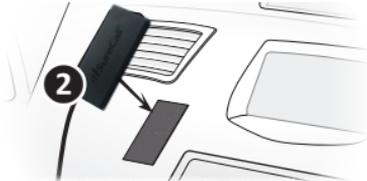
Identify a location for the inside antenna on or near your front dashboard that is: (1) Within 2-3 feet of typical cell phone location, (2) At least 8 inches (20cm) from cellular devices and (3) At least 4 inches (10cm) from metal.
